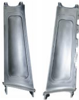
GENx-1B, GE90-Pylon (Aluminium)
